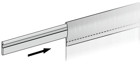
push the prepared panel on the panel profile, the groove should point out to the window side
