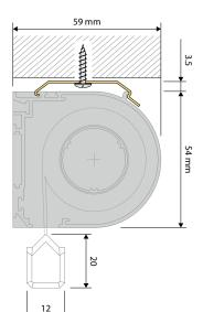
Window sash fixation with profile block holder
