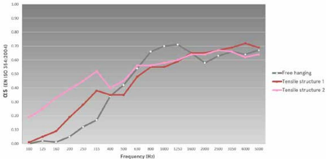
Sound absorption detailed data according to EN ISO 354 available under request
