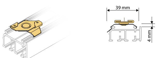
Quick assembly clip with cropped fixing clip for T profile 24–26 mm, only for rails 7620 and 7630
