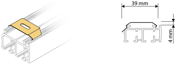
Cropped fixing clip with oval hole for 2 / 3-track rail
