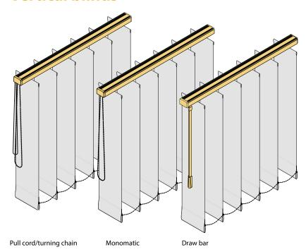
The made to measure vertical blinds consist of aluminium headrails and vertical slats. They can be used in office environments but also in living areas. They are a decorative design element and also provide interior sun control and privacy.
